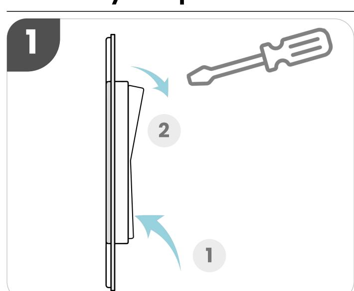
Press and hold the bottom or top of the switch rocker. Use a screwdriver or similar tool to pry the switch rocker off the switch to reveal the battery compartment.
