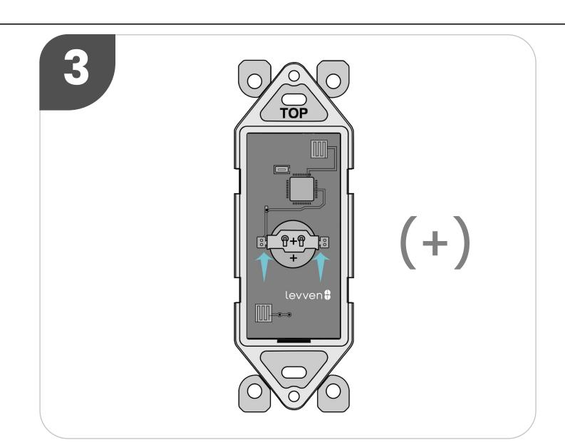
Replace a new battery by pushing it from the bottom of the holder, with the positive (+) symbol facing out. Use ONLY a CR2032 3V 225 mAh lithium coin cell battery.
