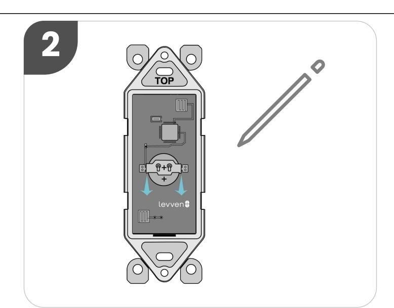
Use a toothpick or similar item to push the battery out of the holder from the top of the holder. Handle the battery as per instructions provided in Important Notes.
