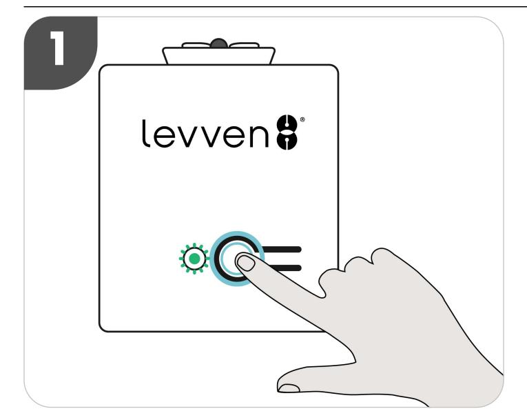
Press and release the pair button on the controller to initiate pairing. This controller's LED will blink green. The pairing mode is active for 60 seconds. If no pairing request is received within 60 secs,
