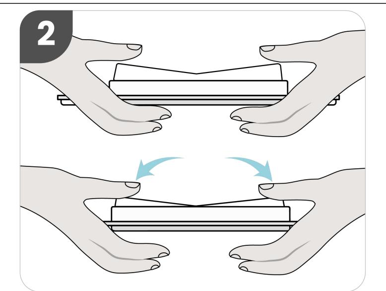
Squeeze and release both ends of the switch simultaneously. Both ends MUST be pressed at the same time to send the pairing signal to the power controller.
