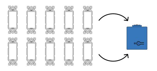
Levven controllers can be paired with up to 10 switches.
