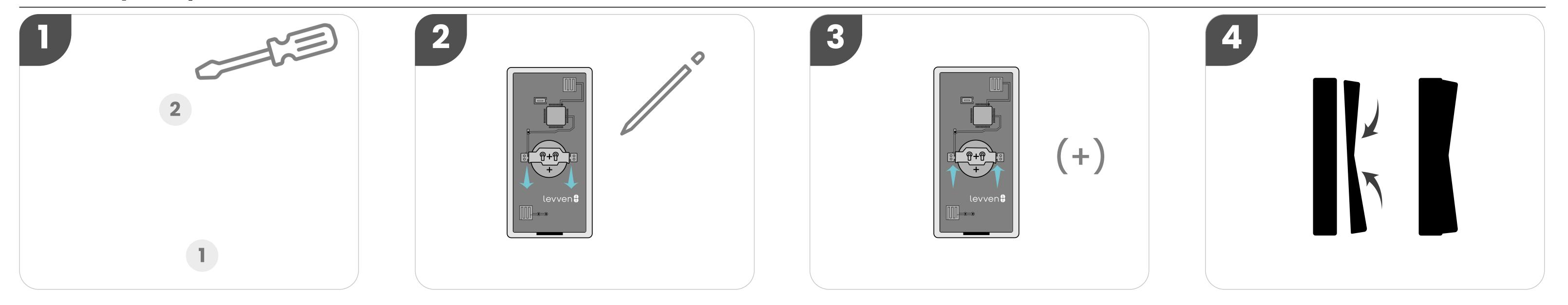
Press and hold the bottom or top of the switch rocker. Use a screwdriver or similar tool to pry the switch rocker off the switch to reveal the battery compartment.
