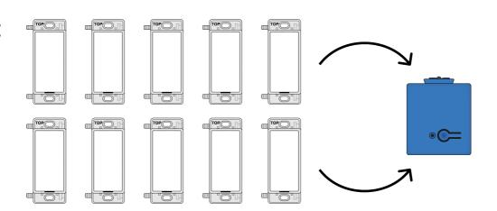
Levven controllers can be paired with up to 10 switches.
