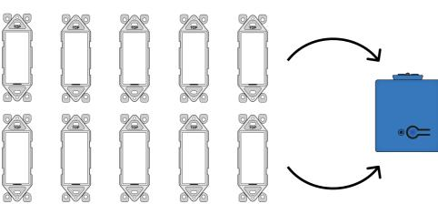
Levven controllers can be paired with up to 10 switches.
